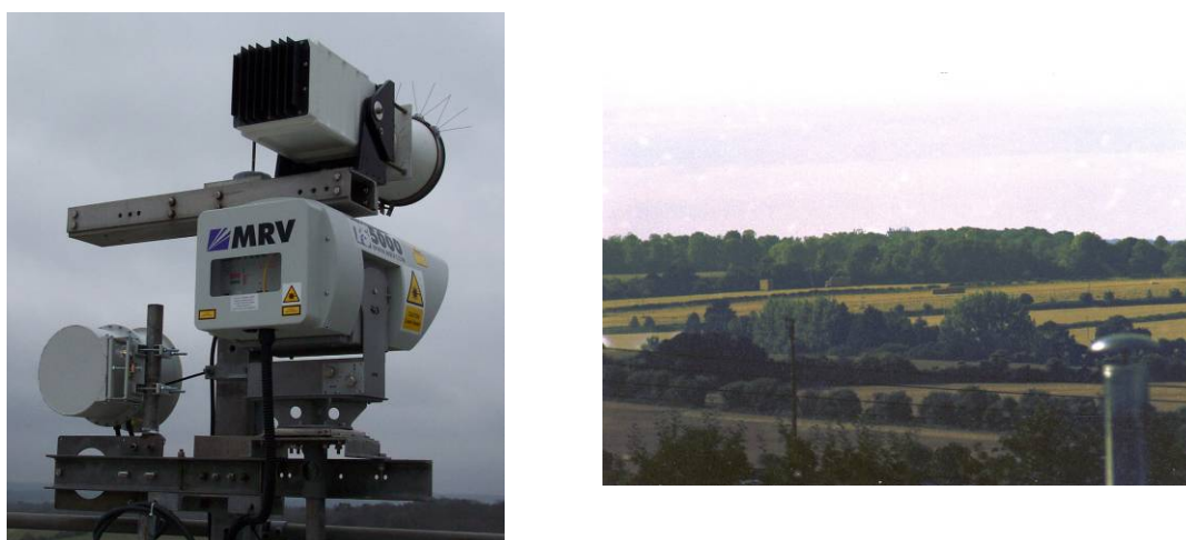
Figure 39: Link transmitters (left) and line of sight path to the receivers (right)
